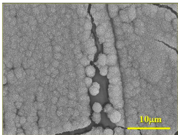
Fig. 1. A typical carbonate apatite layer formed on a bioactive substrate after soaking in Simulated Body Fluid. Image obtained by Dr. J. Juhasz.
