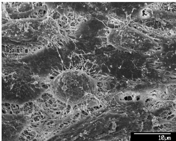
Fig. 4. Osteoblast cells on a glass substrate coating with nanoscale HA deposited via electrohydrodynamic atomisation (image courtesy of Dr. E.S. Thain).
