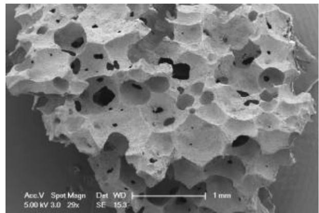
Fig. 2. A hydroxyapatite bone grafting granule. (Sample supplied by ApaTech Ltd.).
