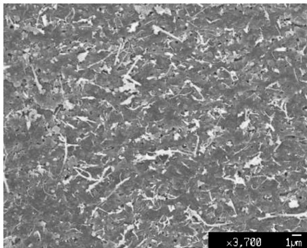
Fig. 5. The surface of a carbon nanotube reinforced HA sample (image courtesy of Ms. A.A. White).
